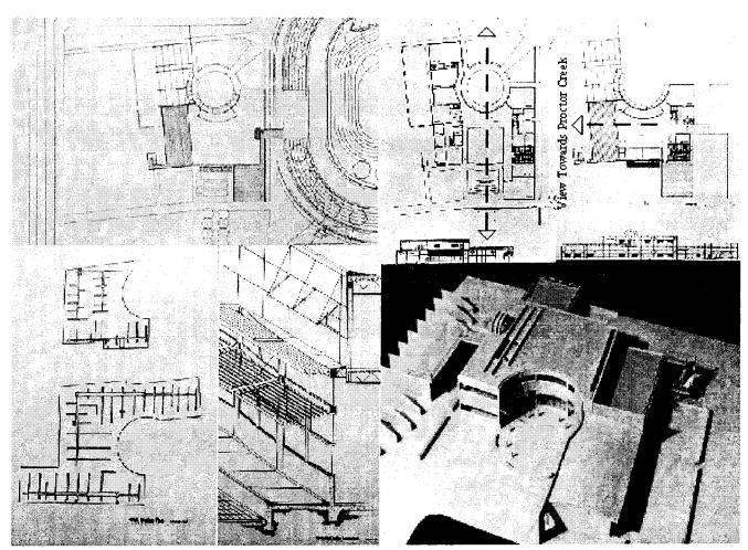
Fig. 4. Community Center 1, (a) Site Plan, (b) First and Second Floor Plans, (c) Duct Layout and South Wall Shading Detail, (d) Building Model (Young Joon Lee, 3rd Arch. Student, Georgia Tech.
